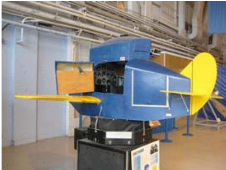
Edwin Link's 'link trainer' flight simulator from 1928 with pneumatic and electrical instrumentation
